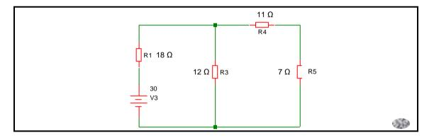
Calculate the current flowing across 12  $\Omega$  using Thévenin's theorem. (8) [12]
